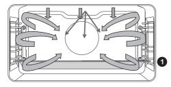
This system uses a combination of microwaves and grill with fan to cut the cooking time.
